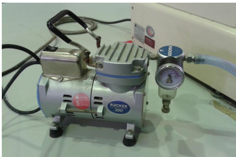
Figure 12: Rocker 300 is used as the source in supplying the suction force to the viscometer for the sample charging process
