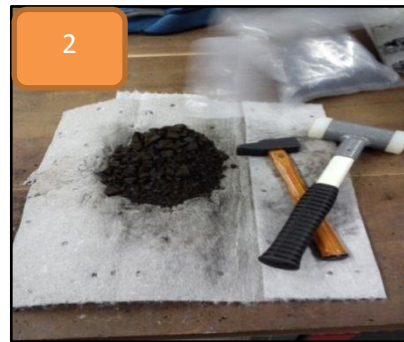
Sample is crashed into finer sizes using hammer
