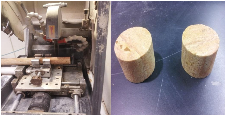
Figure 10: Core being cut into 3cm in height
