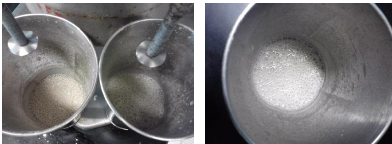
Figure 14: Drilling fluid after mixing
