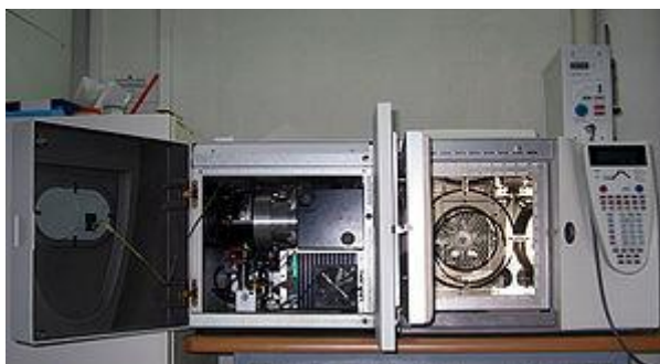
Figure 13: The insides of the GC-MS, with the column of the gas chromatograph in the oven on the right (Wikipedia)
