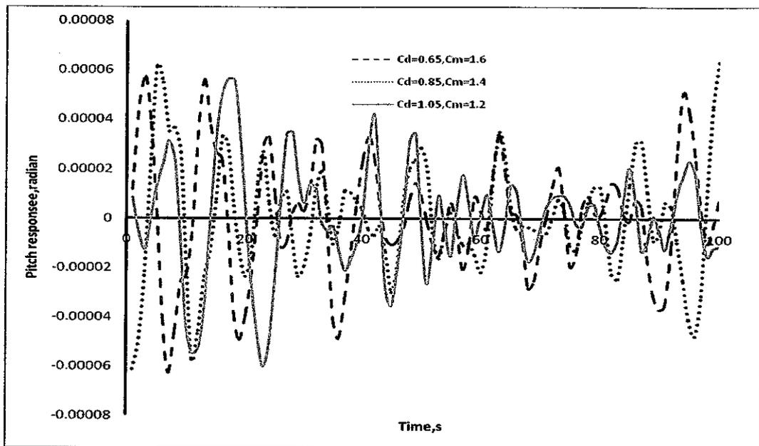
**Figure 4.19:** Graph of Pitch Response subjected to different hydrodynamic coefficients
