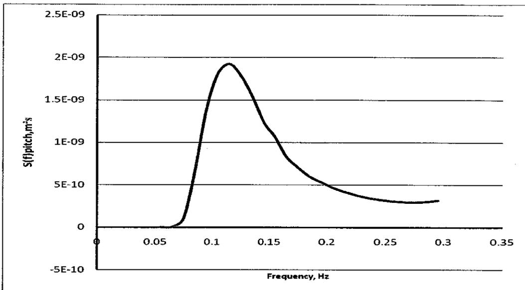
**Figure 4.12:** Graph of surge spectrum,  $S(f)_{PITCH}$  versus frequency
