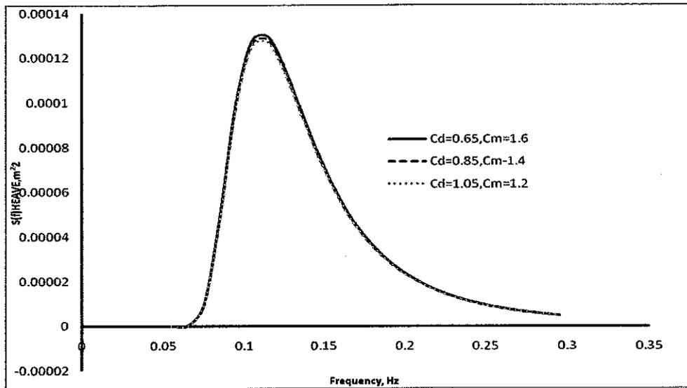
**Figure 4.16:** Graph of Heave spectrum subjected to different hydrodynamic coefficients
