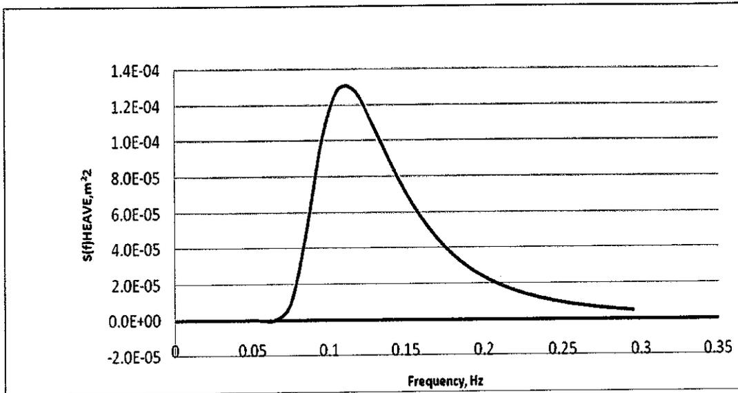
**Figure 4.9:** Graph of heave spectrum,  $S(f)_{HEAVE}$  versus frequency
