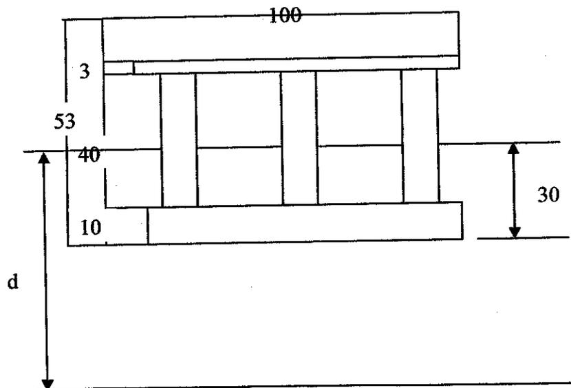
Figure 4.2: Coordinate system for Semi-Submersible Platform from side view
