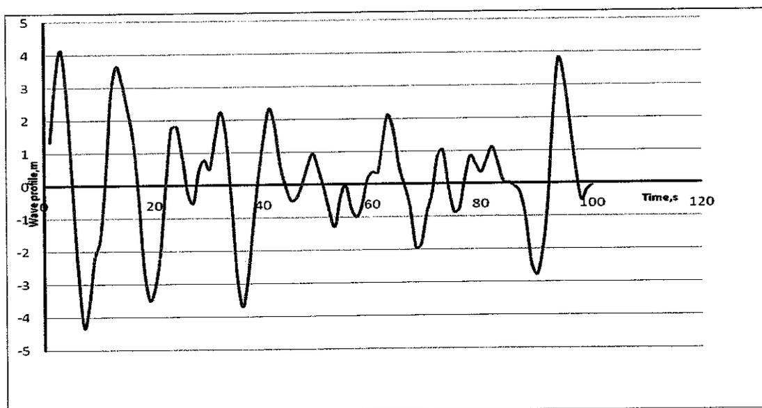
**Figure 4.7:** Graph of surge response at Hull 3 and Hull 4
