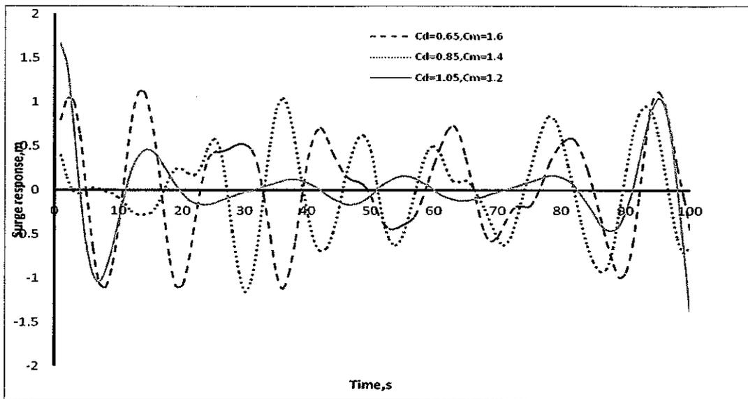
**Figure 4.15:** Graph of Surge Response subjected to different hydrodynamic coefficients
