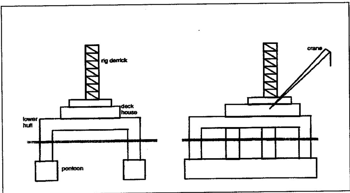
Figure 1.2: Semi-submersible (Yilmaz and Incicek, 1995)
