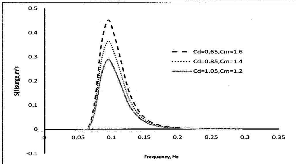
Figure 4.14: Graph of Surge Spectrum subjected to different hydrodynamic coefficients
