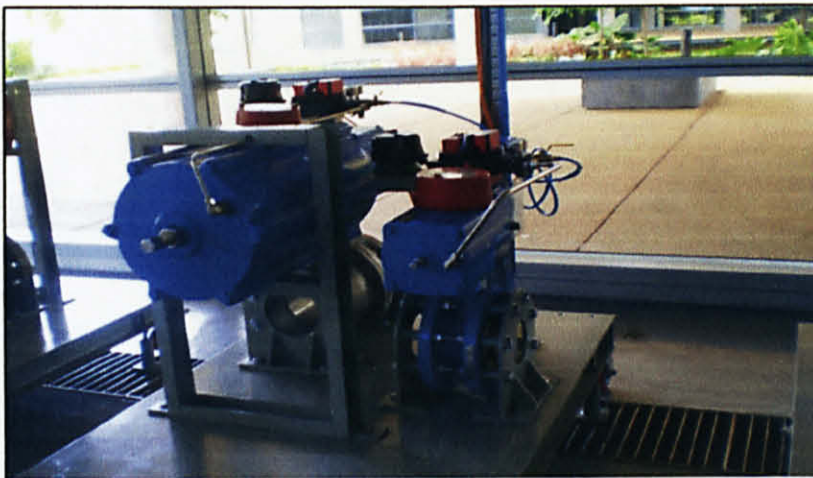
Figure 14: Ball and Butterfly Valve from Metso Neles
