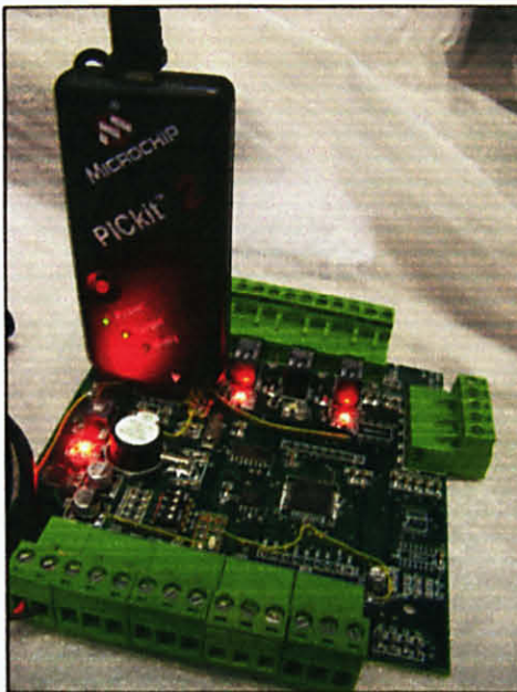
Figure 22 Debugging controller board using PICkit2
