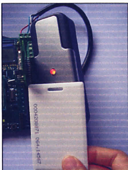
Figure 24 EM card being read by card reader
