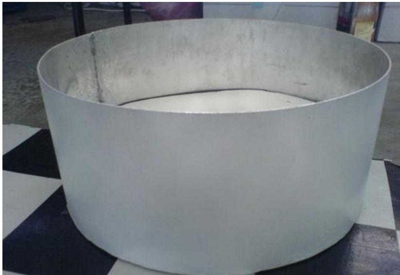
**Figure 25: Scaled Floating Roof Tank Model**
