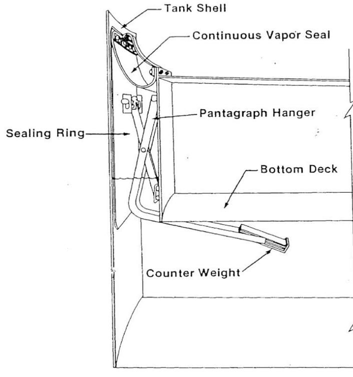
**Figure 4: Roof Seal Component.**
