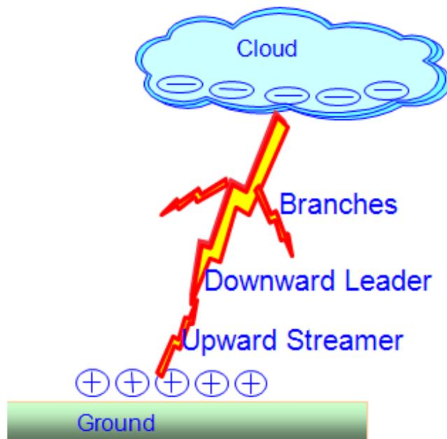
**Figure 7: A Typical Cloud to Ground Lightning.**
