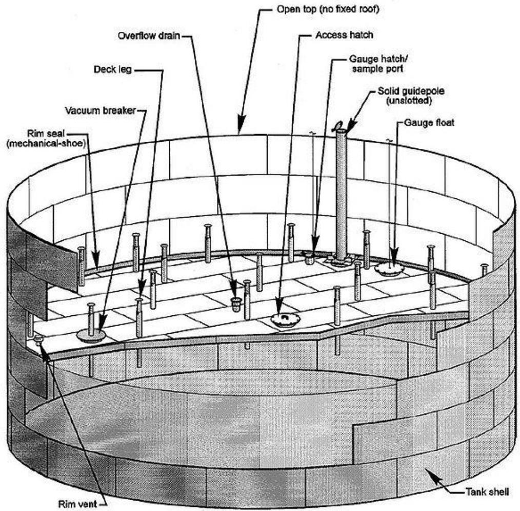
**Figure 2: Floating Roof Tank Components.**
