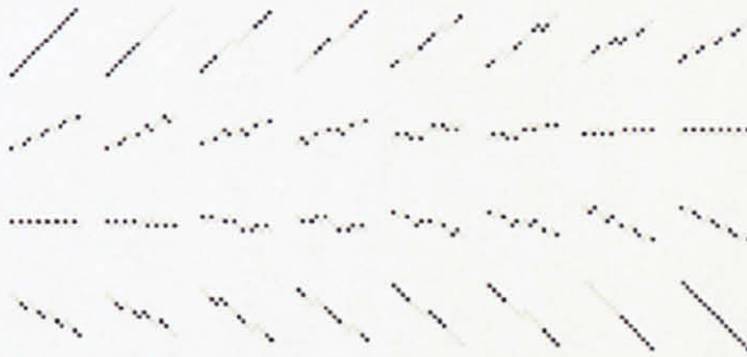
Figure 3: Impulse reponses of 32 directional filters. Those filters correspond to mostly horizontal directions.
