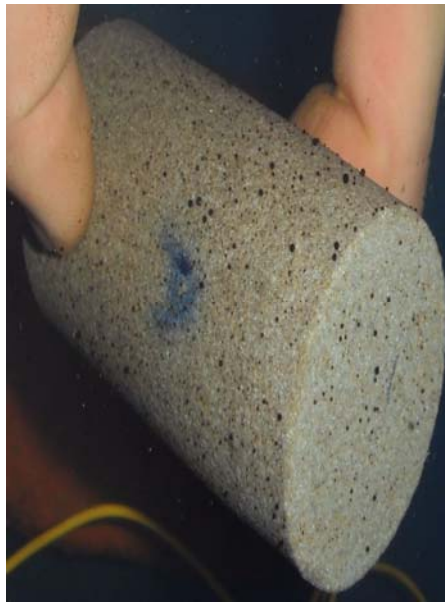
Figure 68: Core sample with More Oil Droplets
