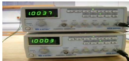
Figure 21: Function generator 5MHz model Instek GFG-8250A
