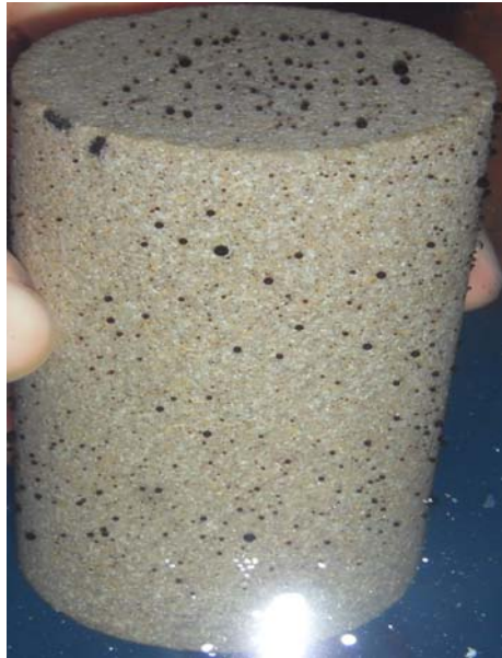
Figure 69: Core Sample with Increasing Number of Oil Droplets
