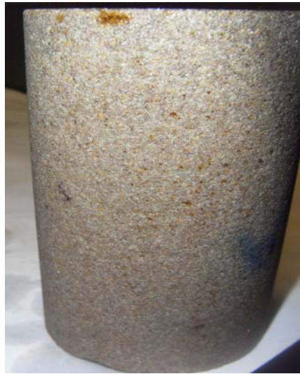
Figure 67: Core Sample with a little oil droplets
