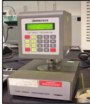
Figure 15: Brookfield Viscometer for Low-Viscosity (LV) type of fluid.
