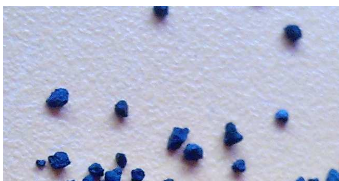
Figure 2.3. Granular Activated Carbon
