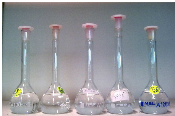
Figure 3.4 : Sample of five different metal concentrations
