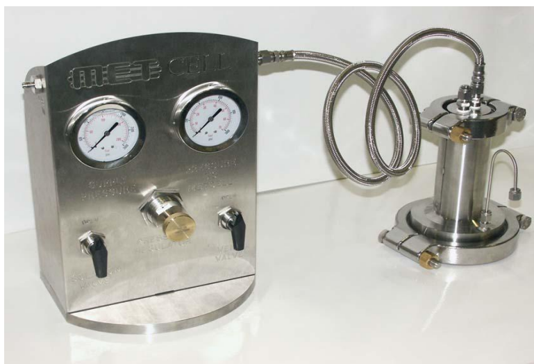
Figure 5: METcell unit and the gas control unit
