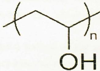
Figure 2.1: Chemical structure of polyvinyl alcohol (PVA)
