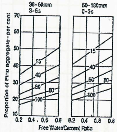
Fig. 14.14 Recommended proportion of fine aggregate (expressed as percentage of total aggregate) as a function of free water/cement ratio for various workability and maximum sizes<sup>14.11</sup> (numbers refer to percentage of fine aggregate passing 800  $\mu$ m sieve) (Building Research Establishment, Crown copyright) (continued on p. 767)
