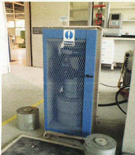
Figure 4.1.3: 2000 kN Compression and Flexural Machine
