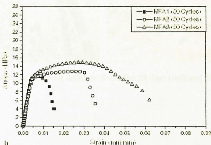
Figure 2.3.4: Stress-strain curves of the composite reinforced with synthetic and cellulose fibers after 50 cycles of accelerated aging test.
