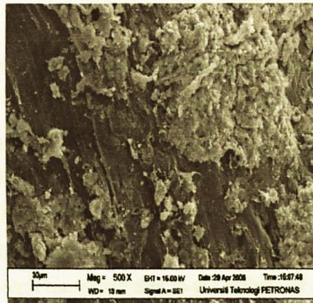
Bonding between PVA fiber and cement after 435 days → 100 X and 500 X zoom
