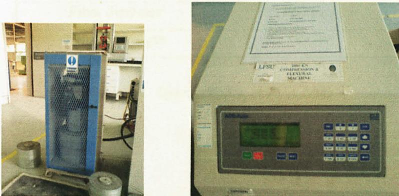
Figure 3.2.3.1: Compression and Flexural Machine
