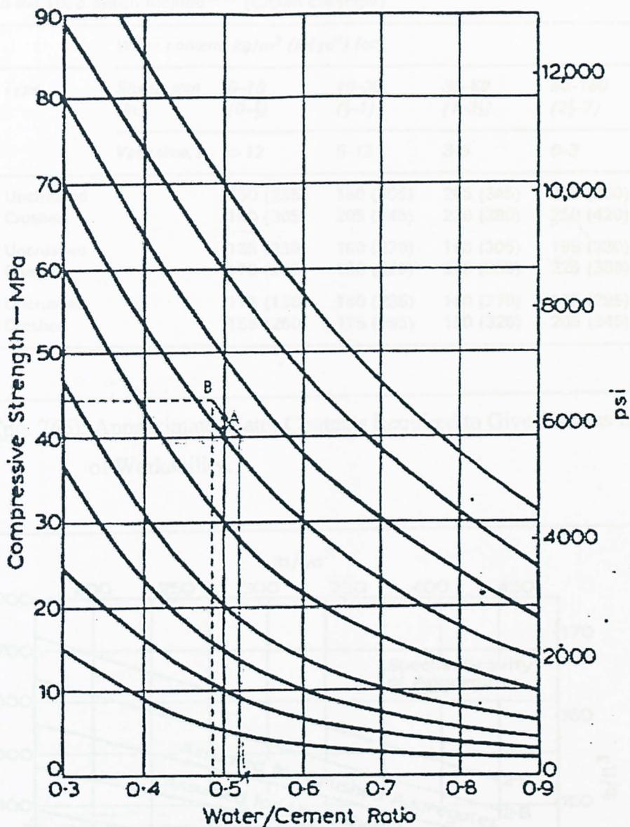
Fig. 14.12 Relation between compressive strength and free water/cement ratio for use British mix selection method<sup>14.11</sup> (see Table 14.9) (Crown copyright)
