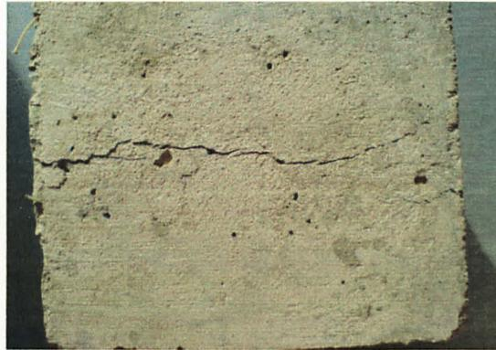
Figure 4.1.2: Line of failure of sample
