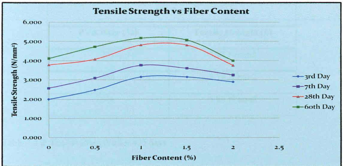
Figure 4.2.3: Tensile strength versus fiber content (2008)
