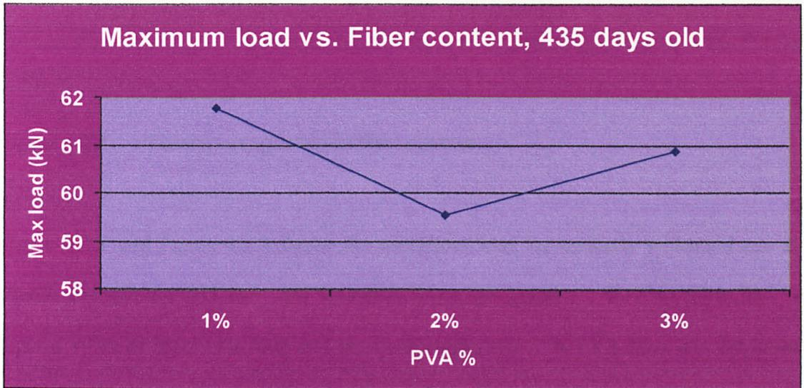
Figure 4.2.1: Maximum load versus fiber content
