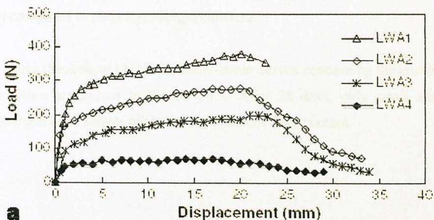
Figure 2.3.1: Load-displacement curves of Fiber Reinforced Concrete
