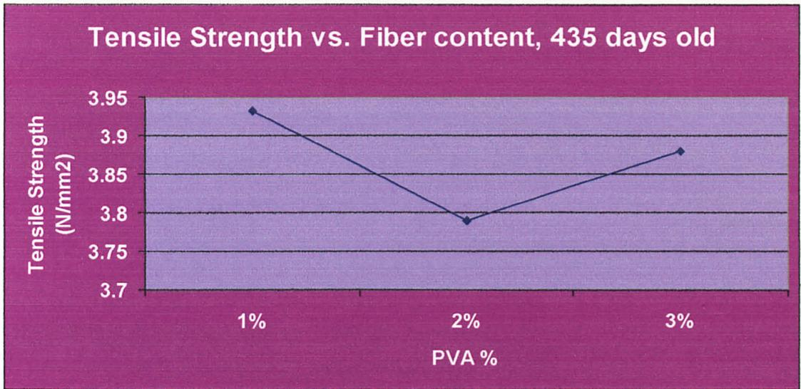
Figure 4.2.2 : Tensile strength versus fiber content
