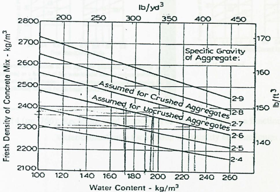
**Fig. 14.13** Estimated wet density for fully compacted concrete<sup>14.11</sup> (specific gravity is given for saturated and surface-dry aggregate) (Crown copyright)
