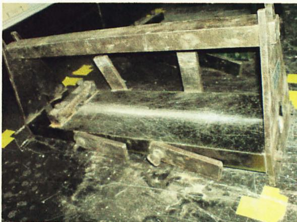
Figure 4.1.1: Cylindrical sample holder for tensile test.
