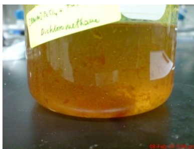
Figure 3 The Oil phase storage ([BMIM]FeCl 4 , PSF and dichloromethane)
