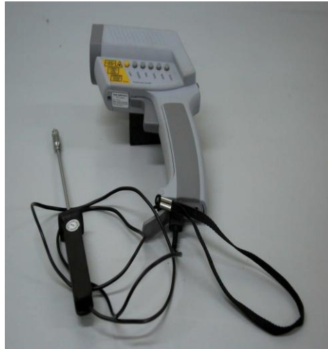
Figure 6 Infrared Pyrometer used by Furnace Operator from OPTIMAL Chemicals (M) Sdn. Bhd to take data in the firebox.
