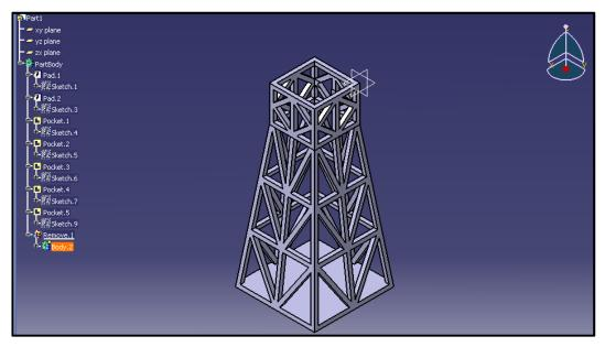
Figure 4.1: Jacket Structure drawing (isometric view) with 1 m x 1 m cross-sectional area of steel members.
