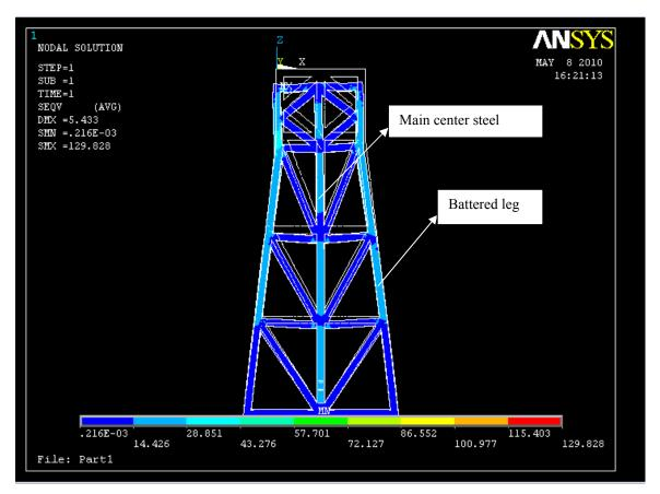
Figure 4.6: Von Mises nodal solution (Contour plot normal view) for Jacket Structure with 1 m x 1 m cross-sectional area steel members at deck load of 200 MN.
