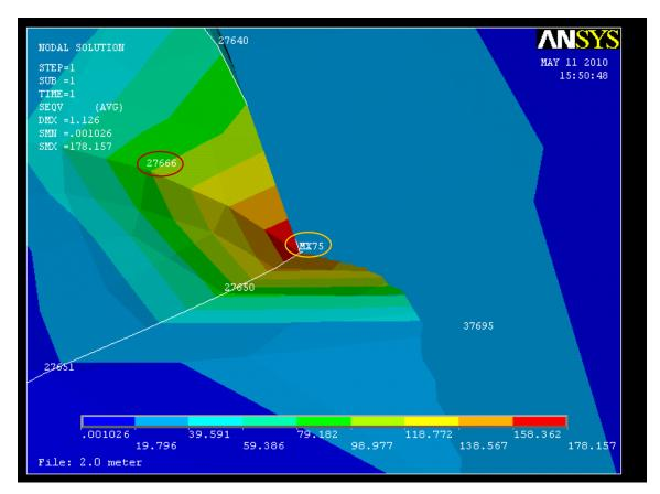
Figure 4.15: Contour plot of nodal solution (node 5175 and 27666) for jacket structure with 2 m x 2 m cross-sectional area steel members at deck load of 200 MN.
