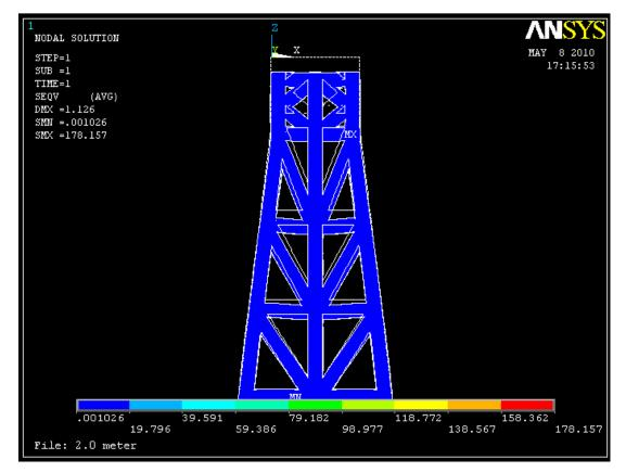
Figure 4.12: Von Mises nodal solution (Contour plot normal view) for Jacket Structure with 2 m x 2 m cross-sectional area steel members at deck load 200 MN.
