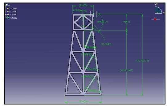
Figure 4.2: Jacket Structure drawing with 1 m x 1 m cross-sectional area of steel members with dimensions.
