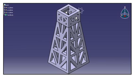
Figure 4.3: Jacket Structure drawing (isometric view) with 2 m x 2 m cross-sectional area of steel members.
