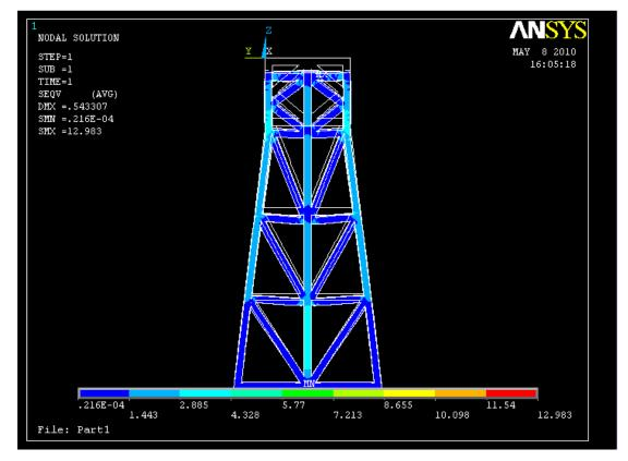
Figure 4.5: Von Mises nodal solution (Contour plot normal view) for Jacket Structure with 1 m x 1 m cross-sectional area steel members at deck load of 20 MN.
