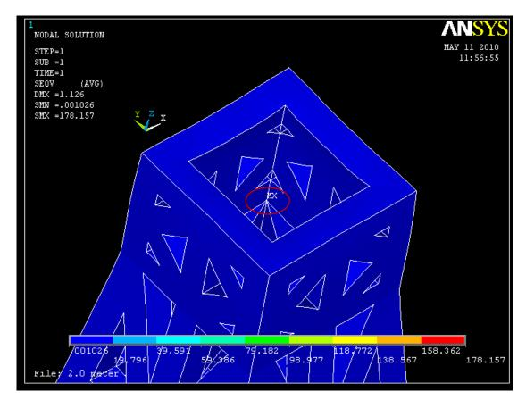
Figure 4.13: Von Mises nodal solution Contour plot (location of SMX) for Jacket Structure with 2 m x 2 m cross-sectional area steel members at deck load of 200 MN.
