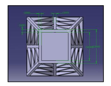
Figure 3.2: Top view of jacket structure of 1 m x 1 m steel members with dimensions.
