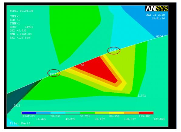
Figure 4.9: Contour plot of nodal solution (node 6055 and 6056) for jacket structure with 1 m x 1 m cross-sectional area steel members at deck load of 200 MN.
