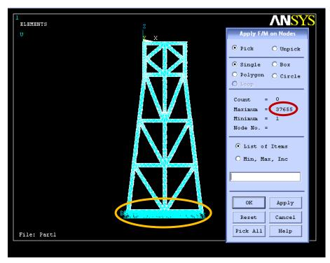
Figure 3.6: Meshed drawing of Jacket structure of 1 m x 1 m cross-sectional area steel members with number total of nodes (marked in red circle).
