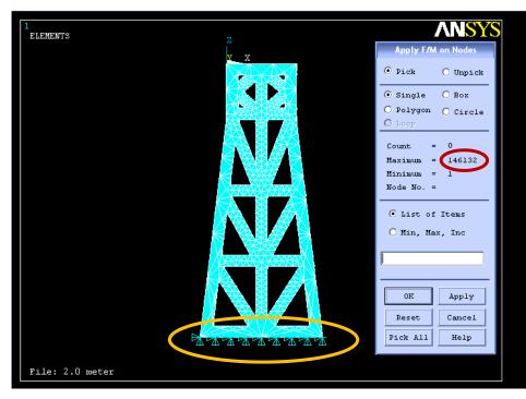
Figure 3.7: Meshed drawing of Jacket structure of 2 m x 2 m cross-sectional area steel members with number total of nodes (marked in red circle).
