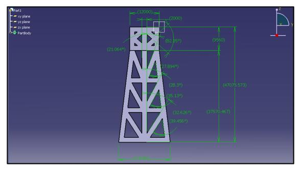
Figure 4.4: Jacket Structure drawing with 2 m x 2 m cross-sectional area of steel members with dimensions.
