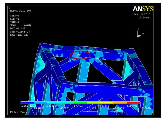
Figure 4.7: Von Mises nodal solution Contour plot (location of SMX) for Jacket Structure with 1 m x 1 m cross-sectional area steel members at deck load of 200 MN.
