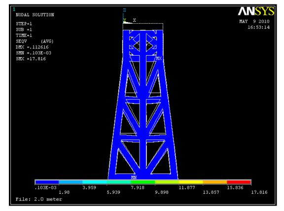
Figure 4.11: Von Mises nodal solution (Contour plot normal view) for Jacket Structure with 2 m x 2 m cross-sectional area steel members at deck load of 20 MN.
