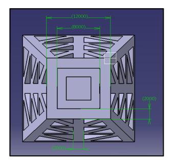
Figure 3.3 Top view of jacket structure of 2 m x 2 m steel members with dimensions.
