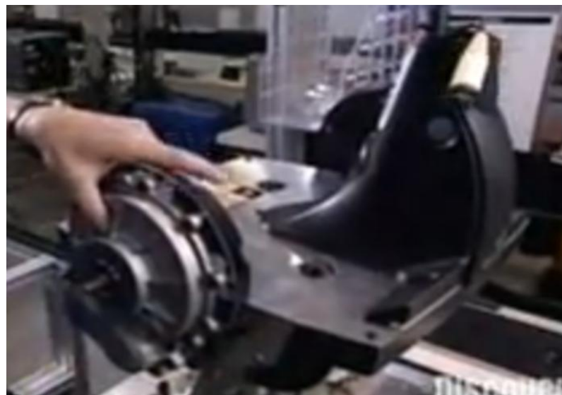
Figure 2.3: Workers install two gearboxes at both sides of Segway-PT main body.
