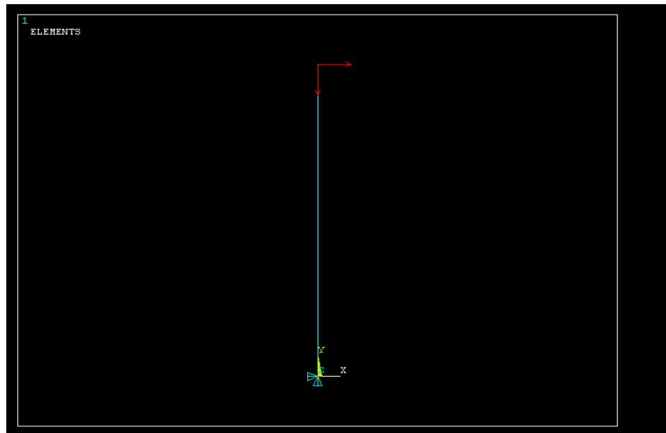
Figure 7: Supporting Condition: Hollow cylinder pinned at the top and fixed at the bottom
