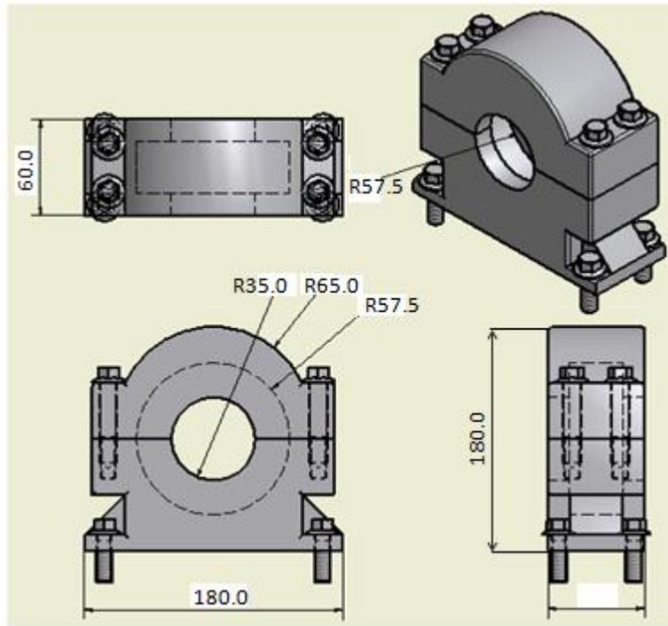
Figure 4.8: projected view of bearing housing
