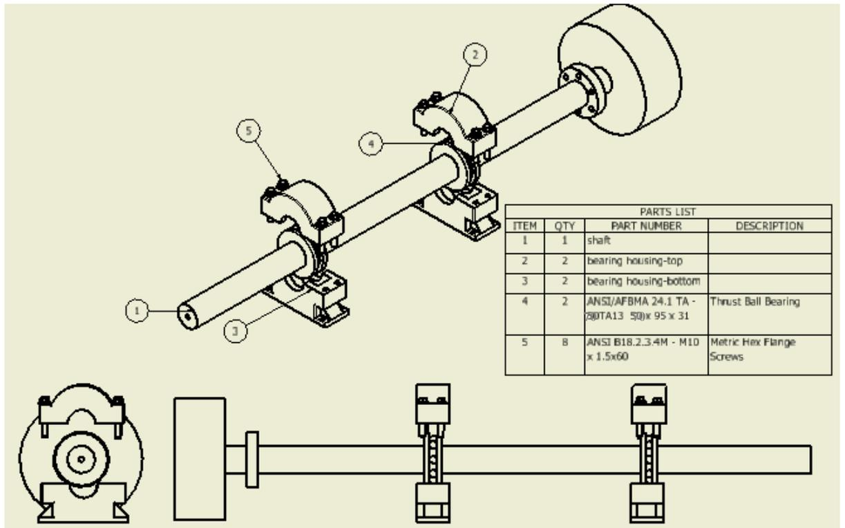
Figure 3.6: 3D view of rig system
