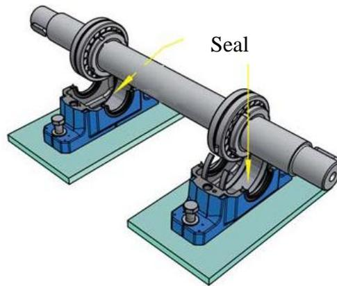
*Figure 4.14: bearing attachment seal*
