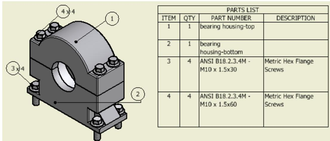
Figure 4.7: base view of bearing housing
