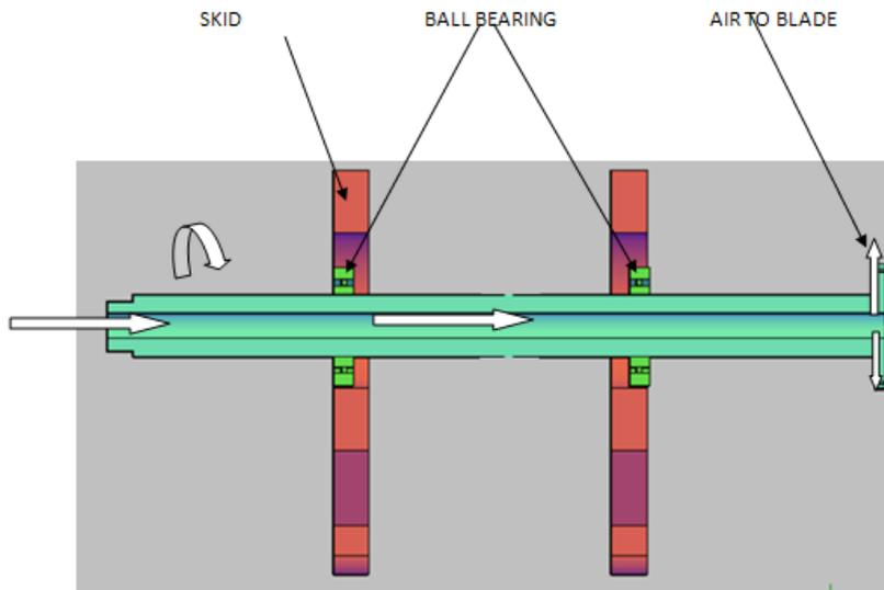
Figure 4.20: flow of air inside the shaft
