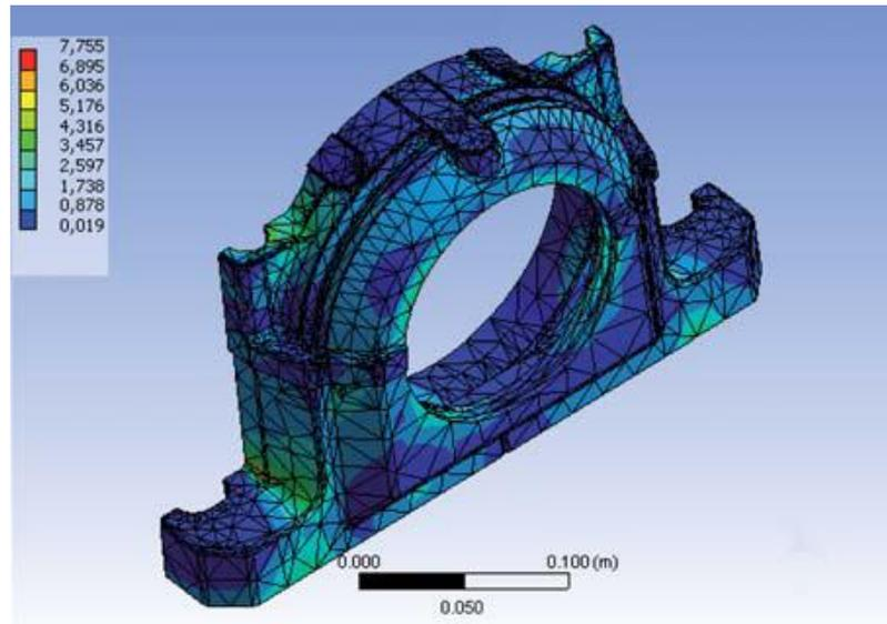
Figure 4.11: analysis of stress on pillow block bearing housing
