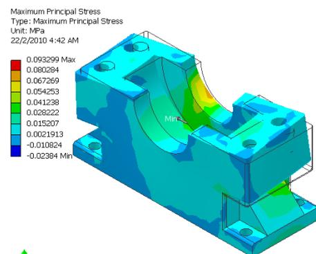
*Figure 4.9: analysis of stress on parts- bottom*
