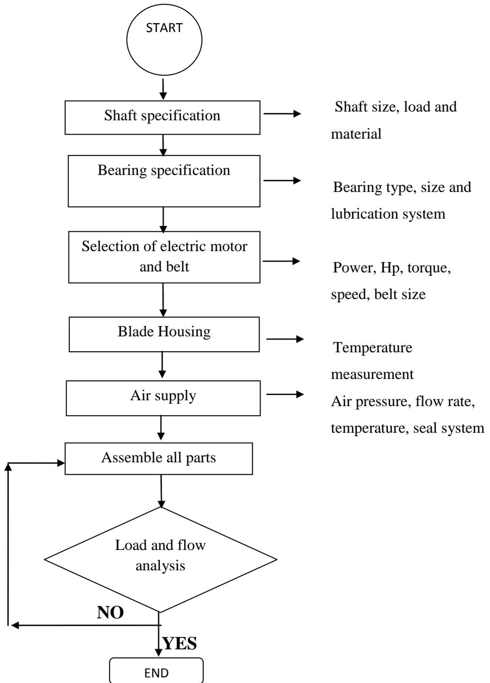
Figure 3.2: flow chart of rig specification development
