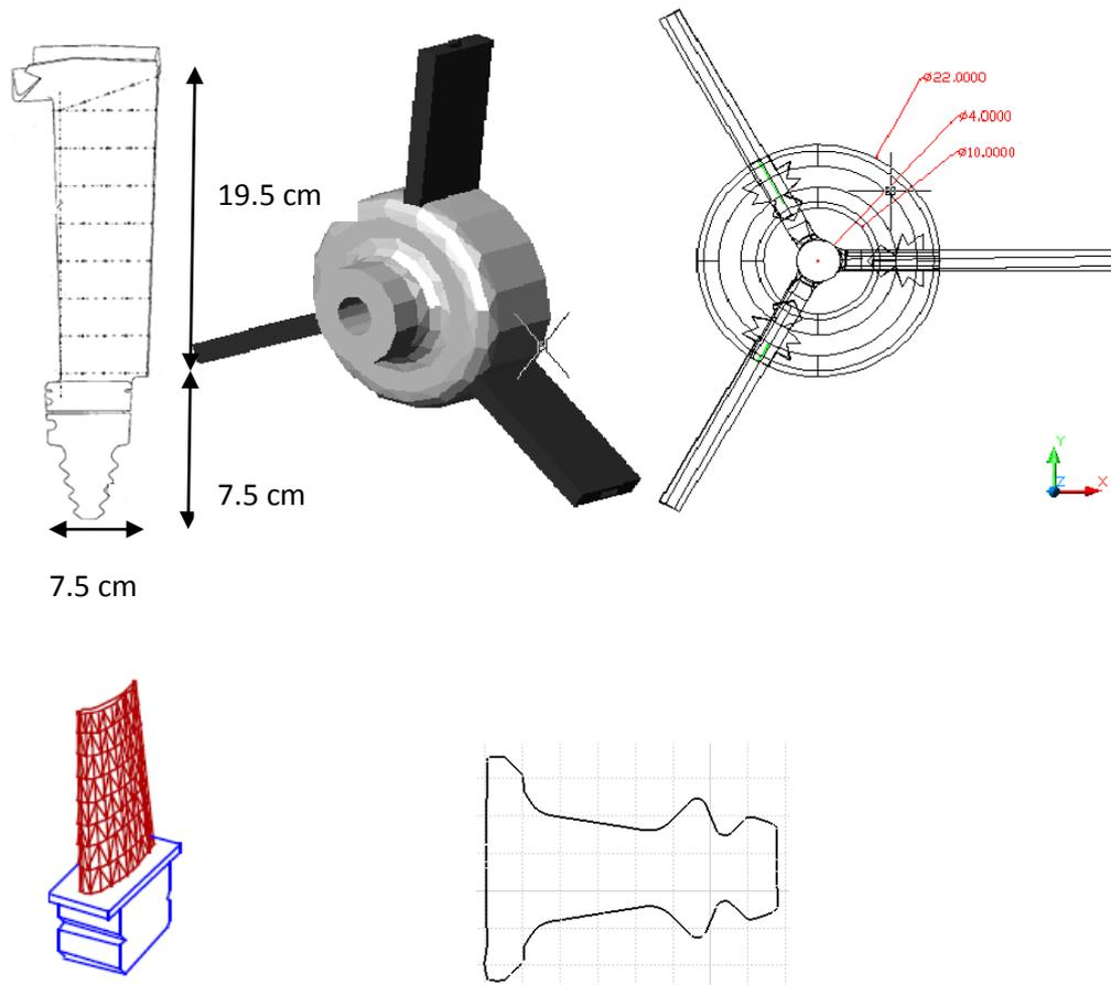
Figure 4.17: blade attachment on flange
