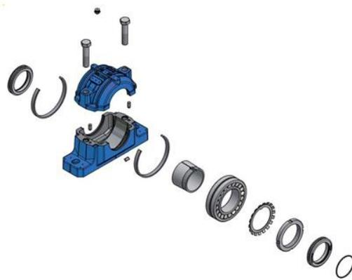
*Figure 4.16: components of the bearing installation on pillow block bearing housing*
