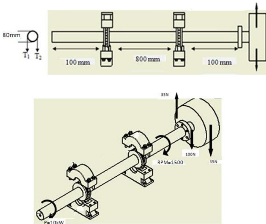
Figure 4.3: shaft diameter calculation
