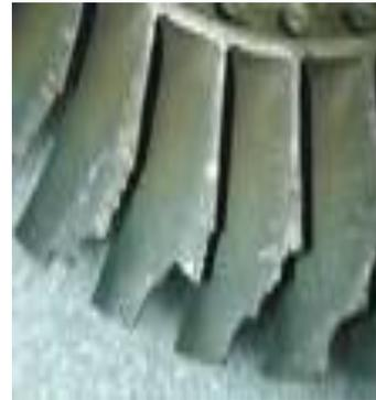
*Figure 1.3 Gas turbine blade damage due to rotation in high temperature and high pressure*
