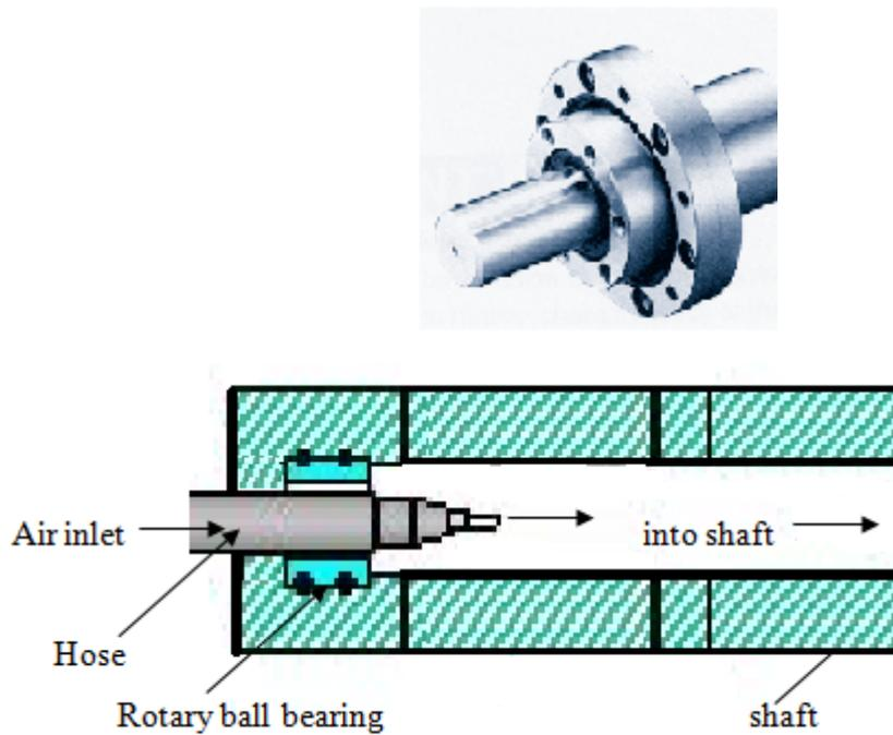
*Figure 4.2: air injection mechanism*
