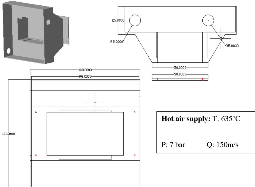
Figure 4.19: hot air and blade housing
