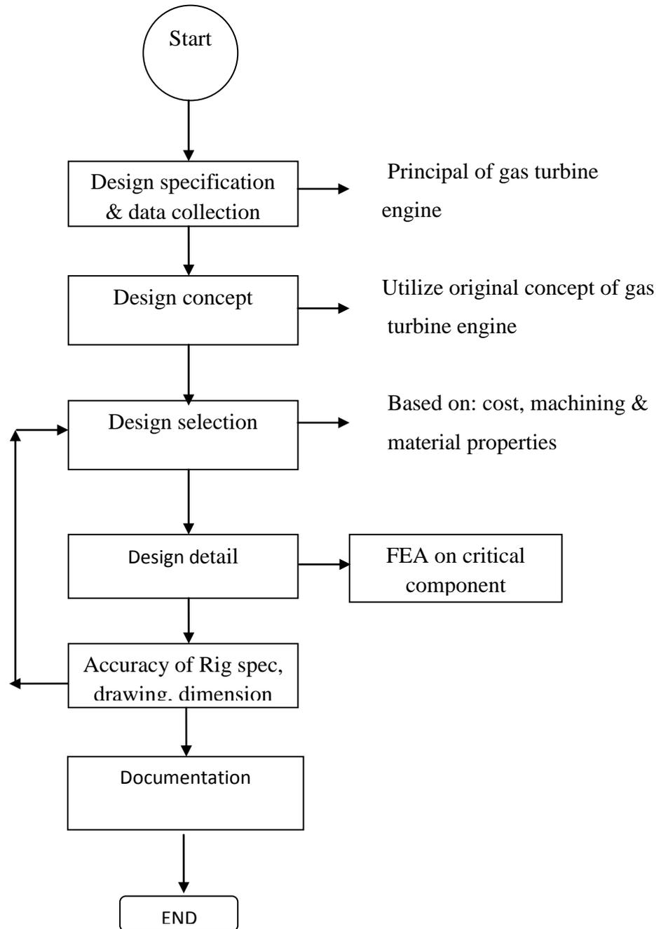
Figure 3.1: Flow chart of test rig development.
