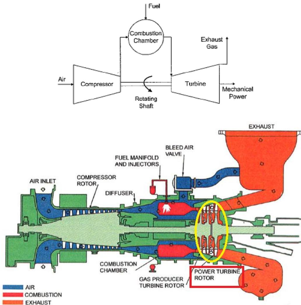
Figure 1.1: gas turbine working principle
