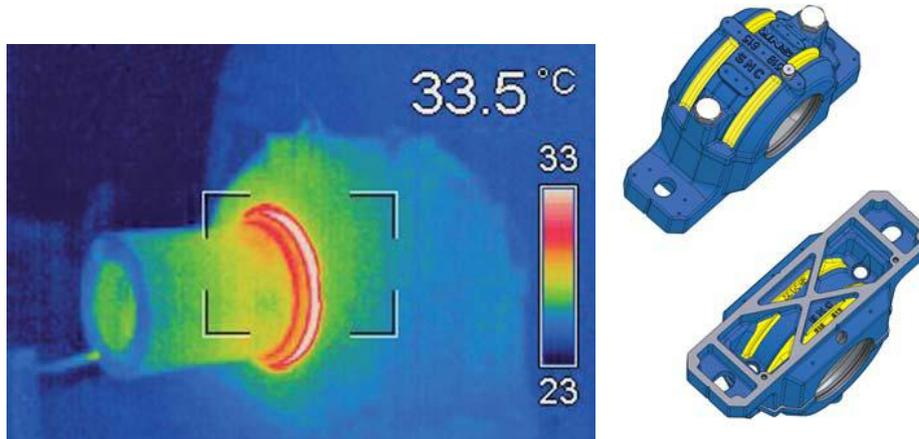
*Figure 4.1.2: analysis of temperature effect on pillow block bearing housing*
