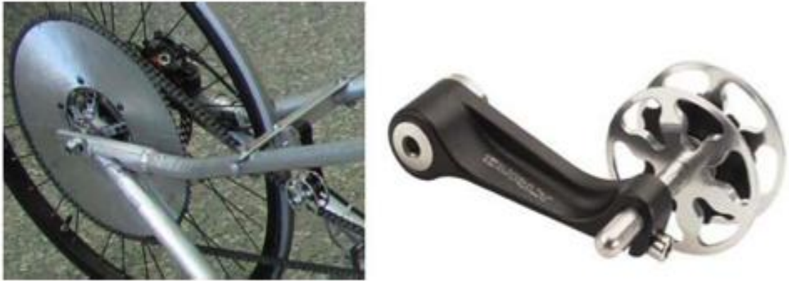
Figure 4.2.5.1: The chain tensioner and the location its been installed
