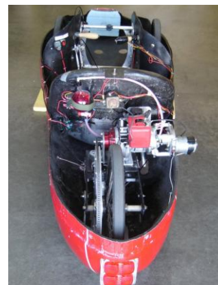
Figure 2.2.4 Linear Transmission (Wheels are directly linked to the engine)
