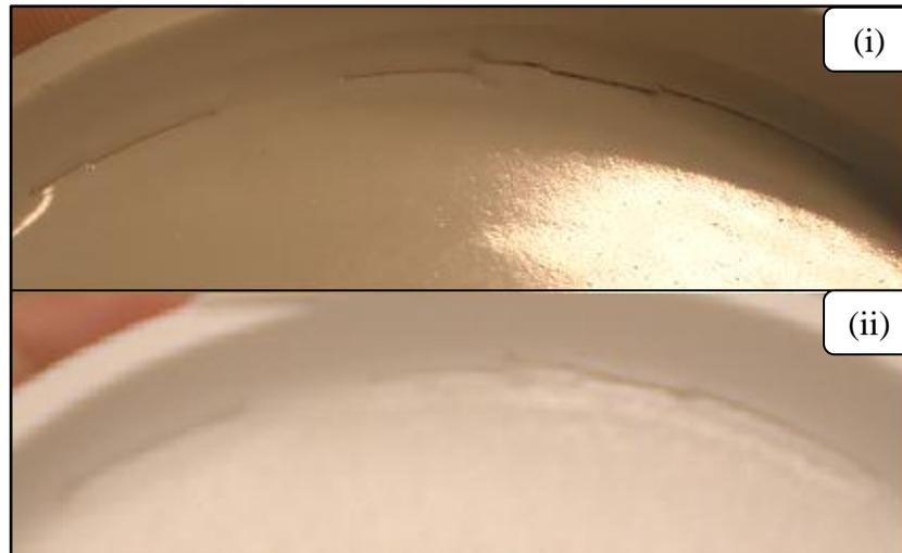
**Figure 21:** Specimen E after Firing at Different Temperatures.
