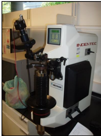
Figure 3.4: Indentec Hardness Testing Machine
