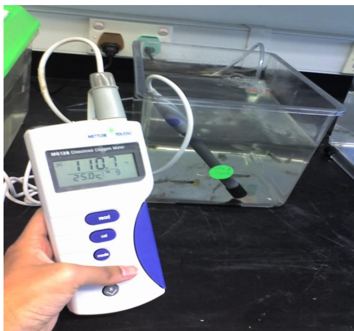
Oxygen dissolved in the water is measured by using dissolved oxygen meter
