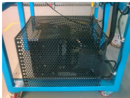
Figure 4.4: ½ HP Refrigerant Chiller.
