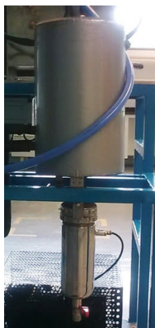
Figure 4.5: From top condenser vessel and below Pyrolysis liquid collection vessel.
