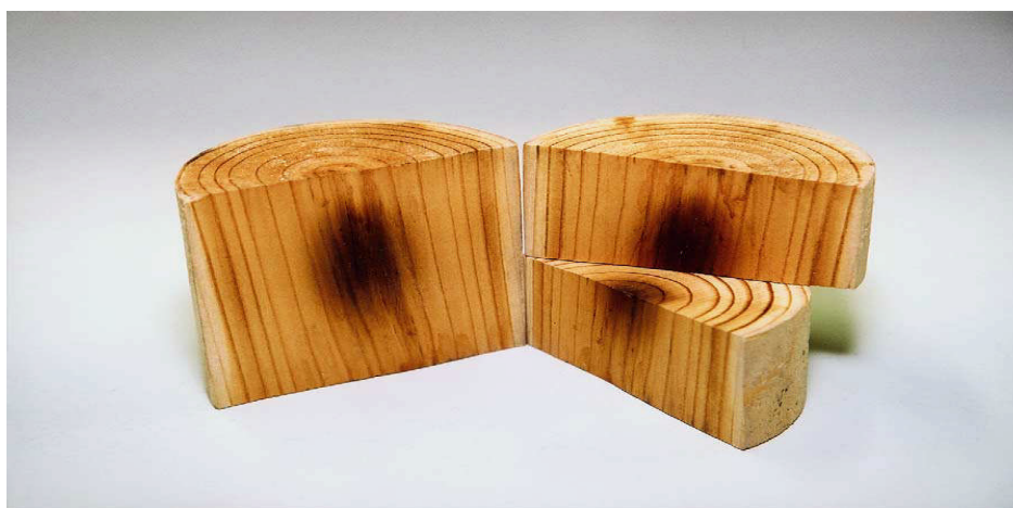
Figure 2.8: Cross-section of wood after 3 minutes of microwave irradiation
