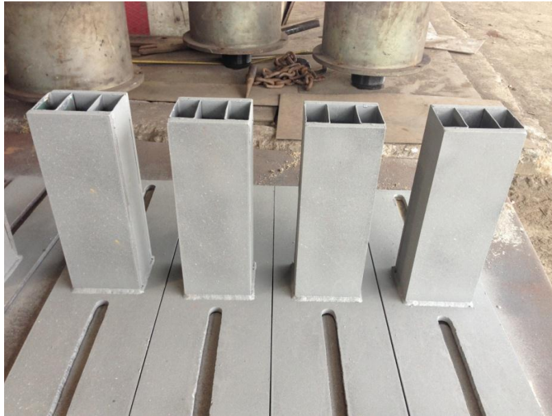
Figure 3.1: Steel blocks after being sandblasted.
