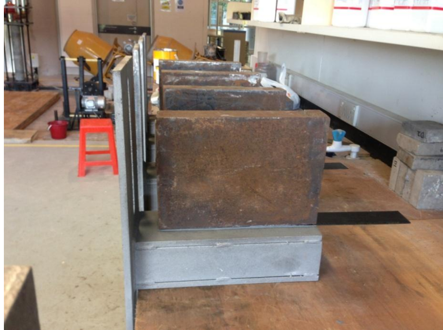
Figure 3.5: Placing weight on top of the CFRP plate.
