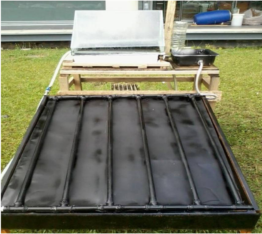
Figure 10: Solar still connected to steel tube collector
