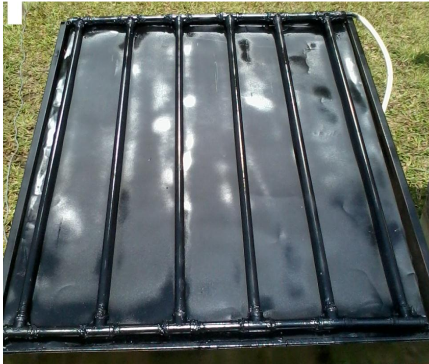
Figure 12: Steel tube system (solar collector)
