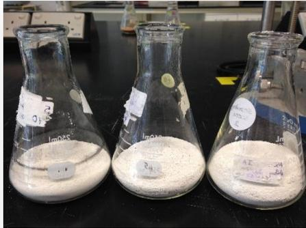
50 gram of samples were mixed with 100mL distilled water
