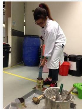
Using a Standard Proctor Hammer
