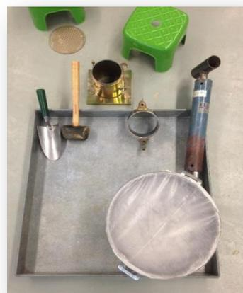
The apparatus that been used for compaction test
