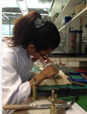
Push the pocket penetrometer until the limit line to obtain the reading
