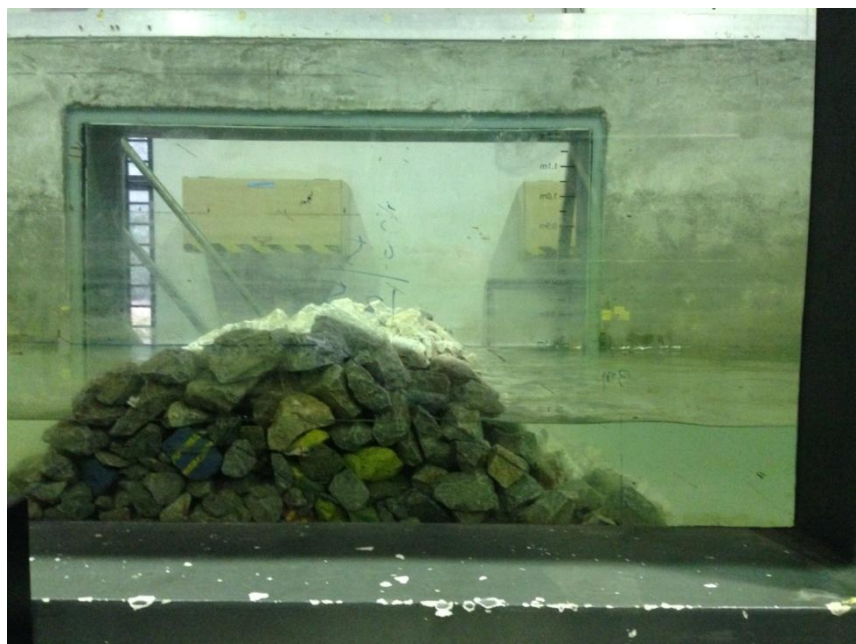
Figure 18 Design cross section of physical breakwater model
