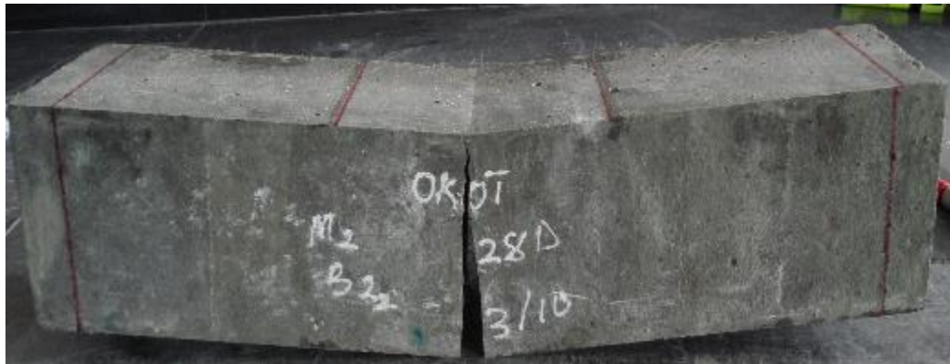
Figure 16 Failure mode of beam sample containing 1% steel fiber
