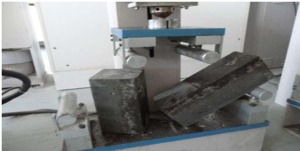
Figure 15 Failure mode of non-fibred beam sample
