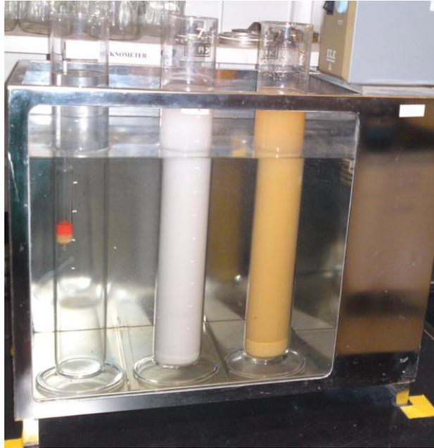
**Figure A-4: The barite solutions contained by sedimentation cylinder being put in 24°C water bath.**
