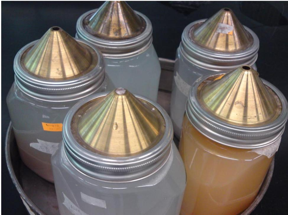
Figure A-1: Pyknometers being filled with barite solutions during the experiment.
