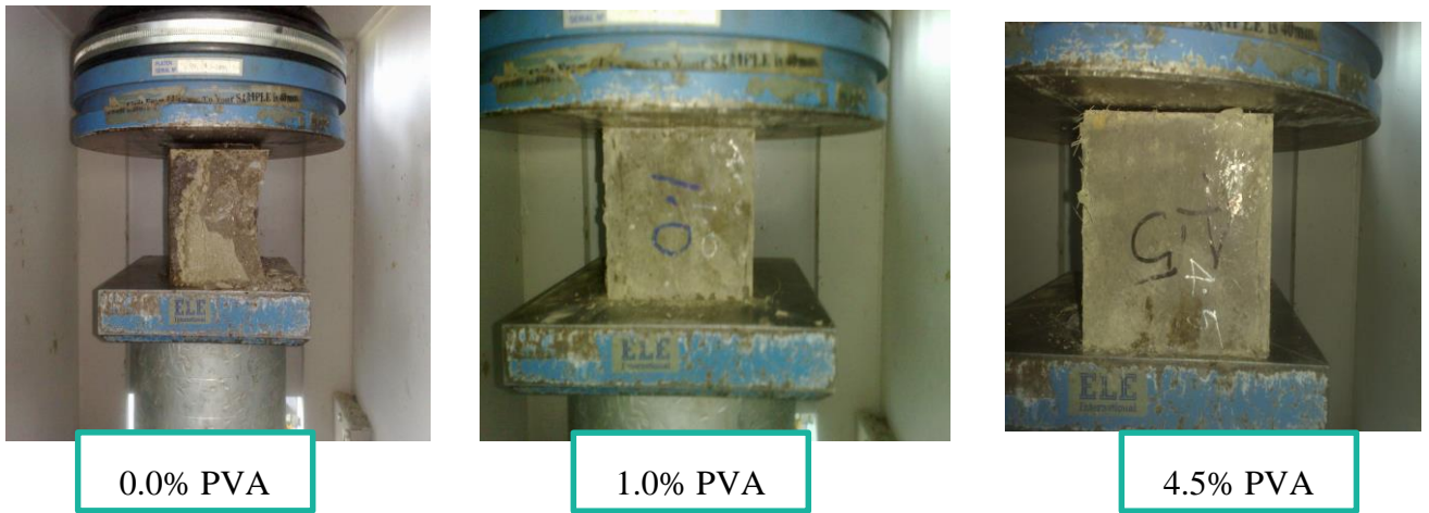
Figure 4.10: Compressive strength test result for different percentage of PVA.
