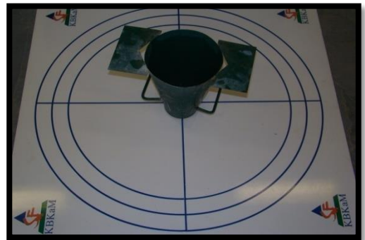
Figure 3.8: Slump flow T500mm in diameter
