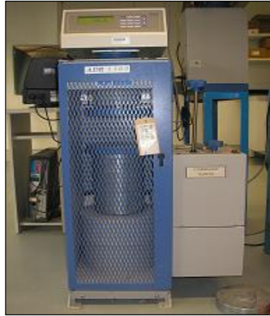
Figure 3.12: Compression machine (ADR 1500)
