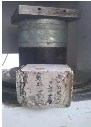
Figure 6: Sample under compression test
