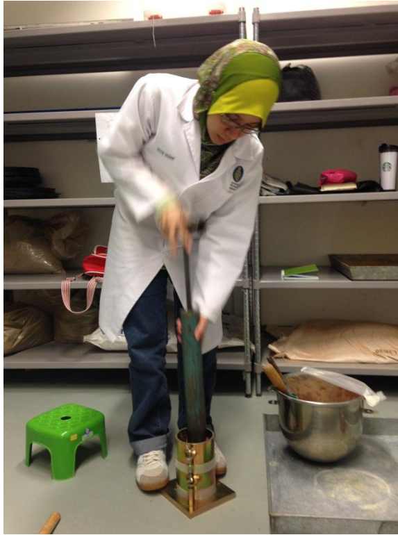
1) Sample was compacted layer by layer by using a Standard Proctor Hammer
