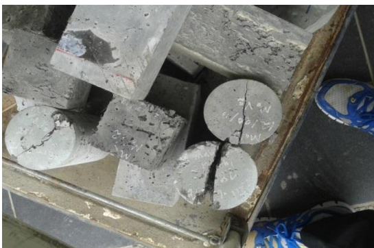
CONCRETE AFTER TESTED
