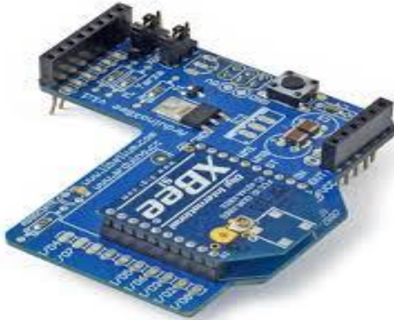
Figure 8: ZigBee Transmitter Part
