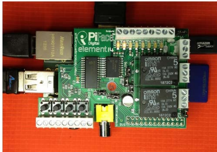
Figure 12 Interfacing with Raspberry Pi and Pi Face
