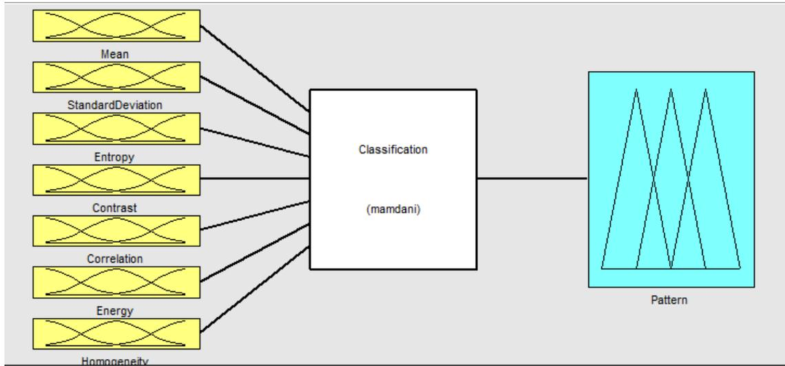
Figure 7: Input and output to the fuzzy inference system
