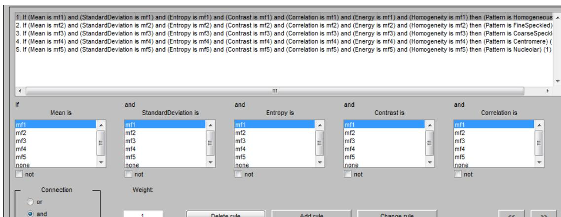
Figure 10: Rule-based structure for fuzzy logic
