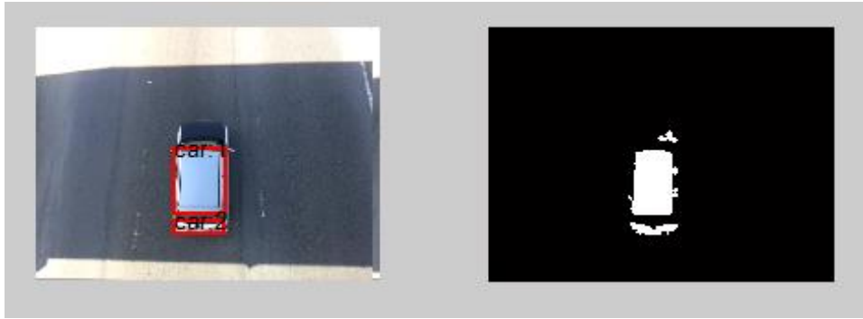
Figure 9: Background Subtraction of passing vehicle
