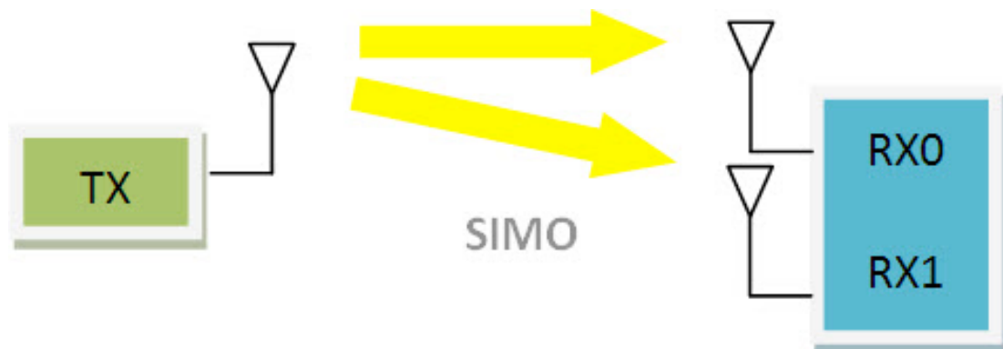
Figure 1: The transmission mode of SIMO (single input multiple outputs)
