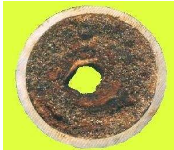
Figure 1-1 Wax deposits in pipelines [3]
