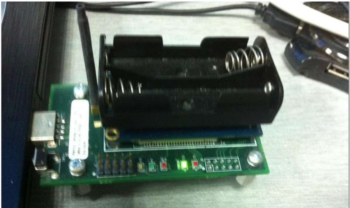
Figure 16: Assembled MIB520 Interface board with IRIS mote
