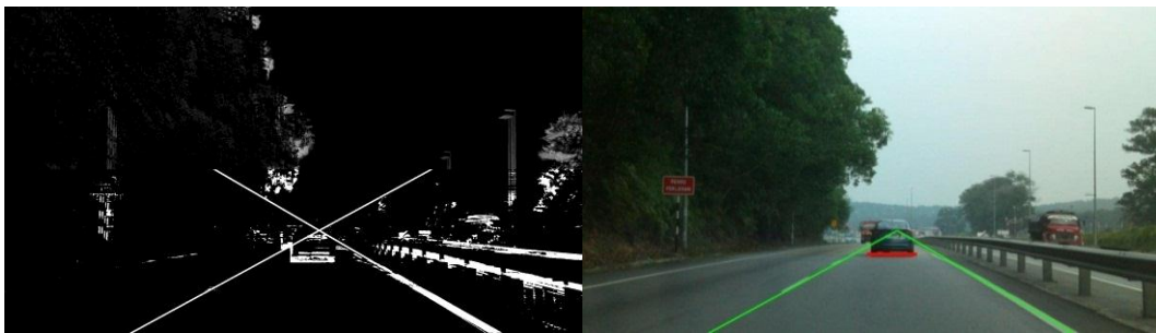
Figure 26: Detected Road Markings from Image Sequence 56-60 (Left), Detected Vehicle in Image 60 (Right)
