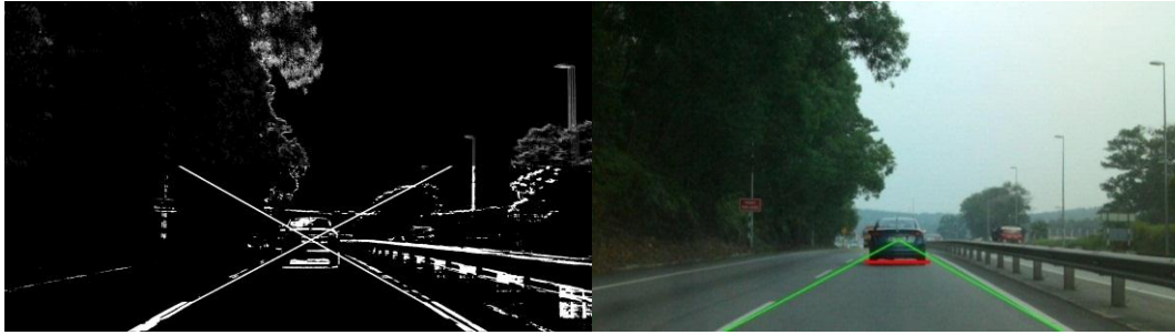
Figure 25: Detected Road Markings from Image Sequence 22-26 (Left), Detected Vehicle in Image 26 (Right)
