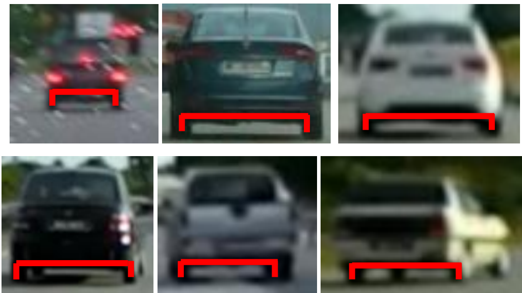
Figure 10: Inverted U-shape Back Wheel Structure of Several Vehicles
