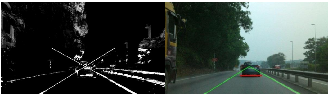
Figure 23: Detected Road Markings from Image Sequence 1-5 (Left), Detected Vehicle in Image 5 (Right)
