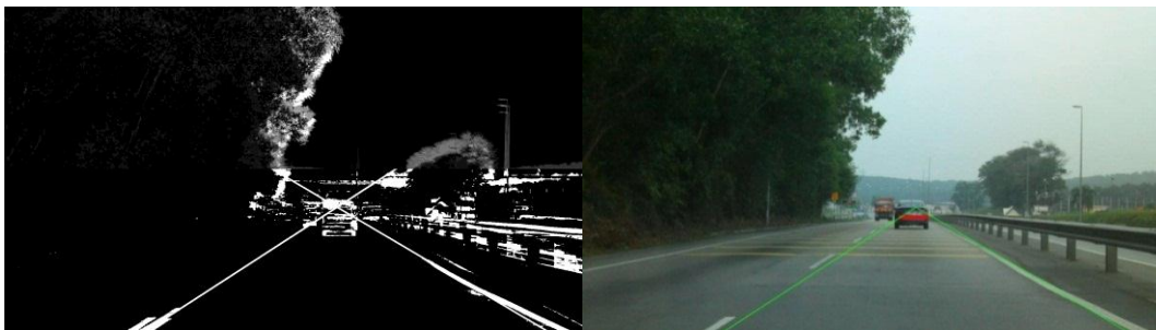
Figure 27: Detected Road Markings from Image Sequence 98-102 (Left), Detected Vehicle in Image 102 (Right)
