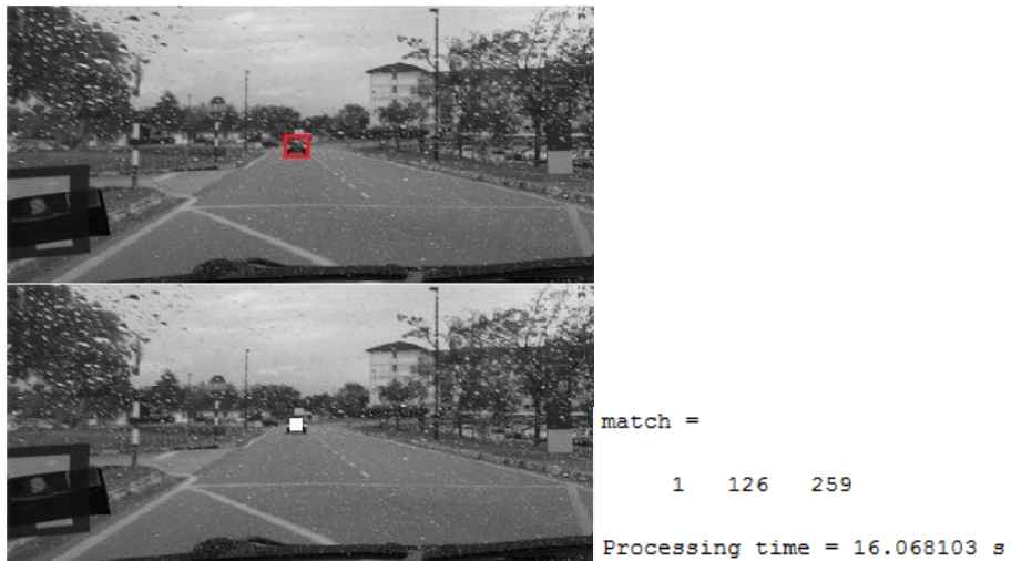
Figure 20: Detected Target (White Box) Using Template Extracted (Red Box) from Original Image
