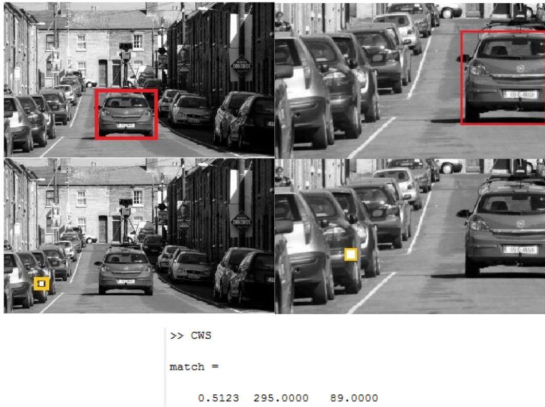
Figure 22: Inaccurate Object Detection due to Undersize Template: Expected Object (Red Box) & Inaccurate Detected Object (Yellow Box)
