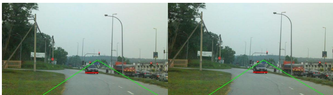
Figure 28: Detected Vehicle Approaching from Front
