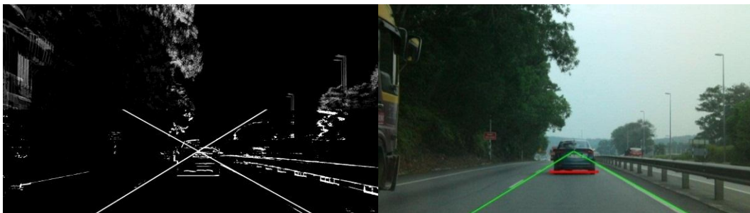
Figure 24: Detected Road Markings from Image Sequence 7-11 (Left), Detected Vehicle in Image 11 (Right)
