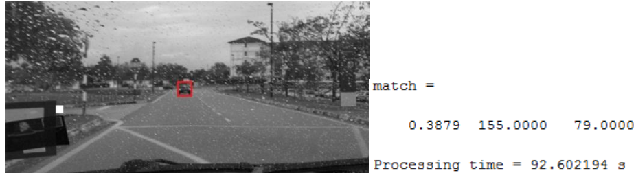
Figure 18: Detected Object (White Box) vs Targeted Object (Red Box)
