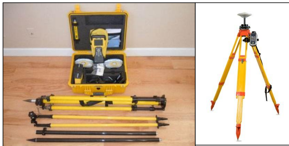
Figure 3.4.1. The RTK GPS Hardware Equipments.
