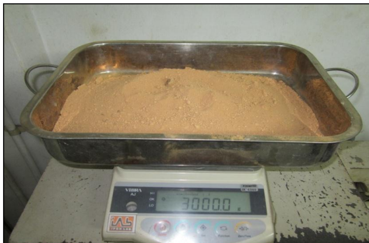
Figure 7: Soil sample are weighed about 3000g
