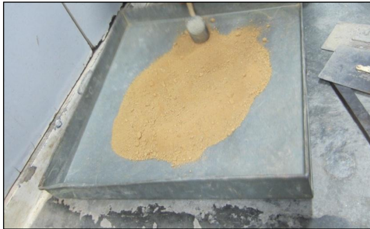
Figure 6: The sample is crushed using a rubber hammer
