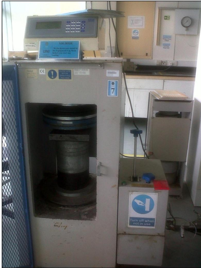
Figure 3.3 Compressive Strength Machine
