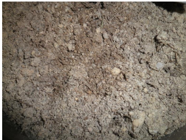
Figure 14 Oven-dried soil with 5% moisture content
