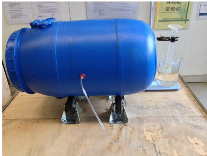
Figure 6 Experimental Set Up at the laboratory; The red circle shows the gas outlet
