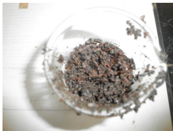
Figure 10 A sample taken from the compost reactor which consists of oil sludge, coir and poultry manure
