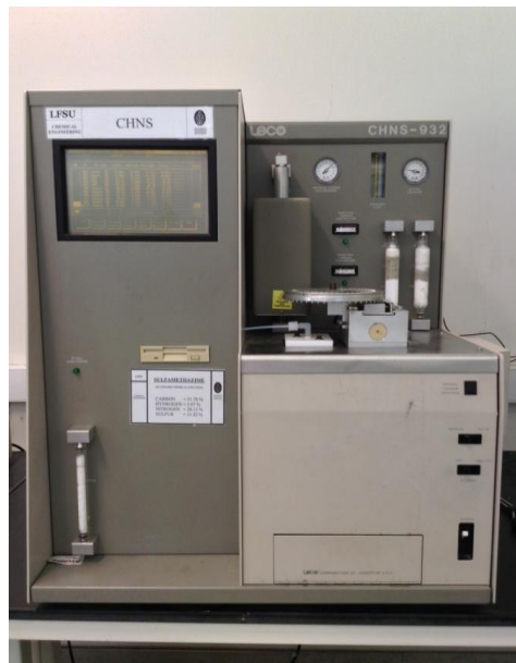
Figure 7 CHNS Analyzer used to analyzed the carbon and nitrogen content of the poultry manure, oil sludge, palm fronds and coir
