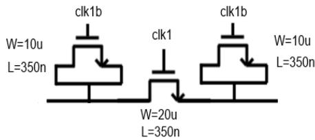
Figure 16, NMOS Switch with Dummies for Charge Injection Compensation
