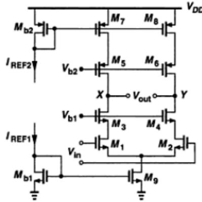
Figure 12: Reference Telescopic Cascode Op-Amp Structure[11]
