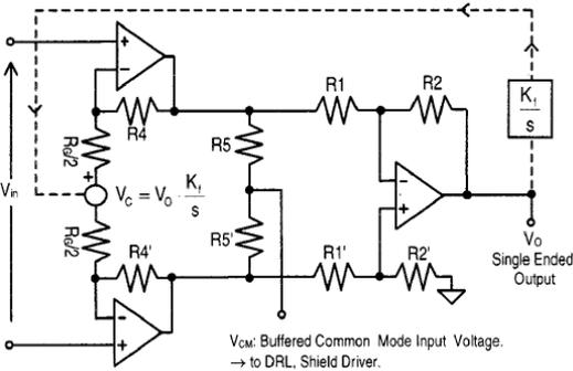
Figure 5: Three op-amps structure proposed by [18].
