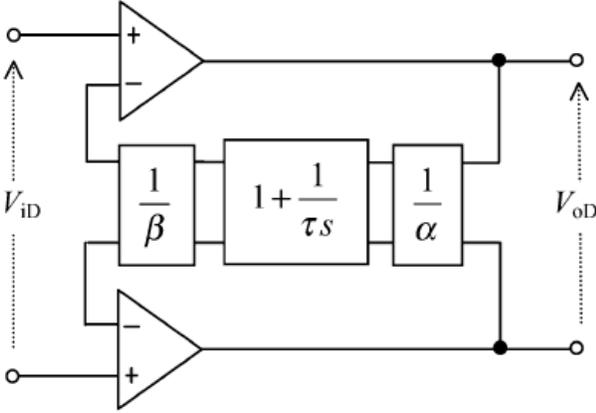
Figure 6: Simplified output DC feedback proposed by [19]
