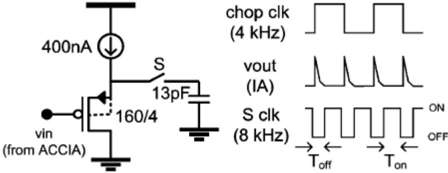
Figure 3: Chopping Spike Filter with its principle operations [5]
