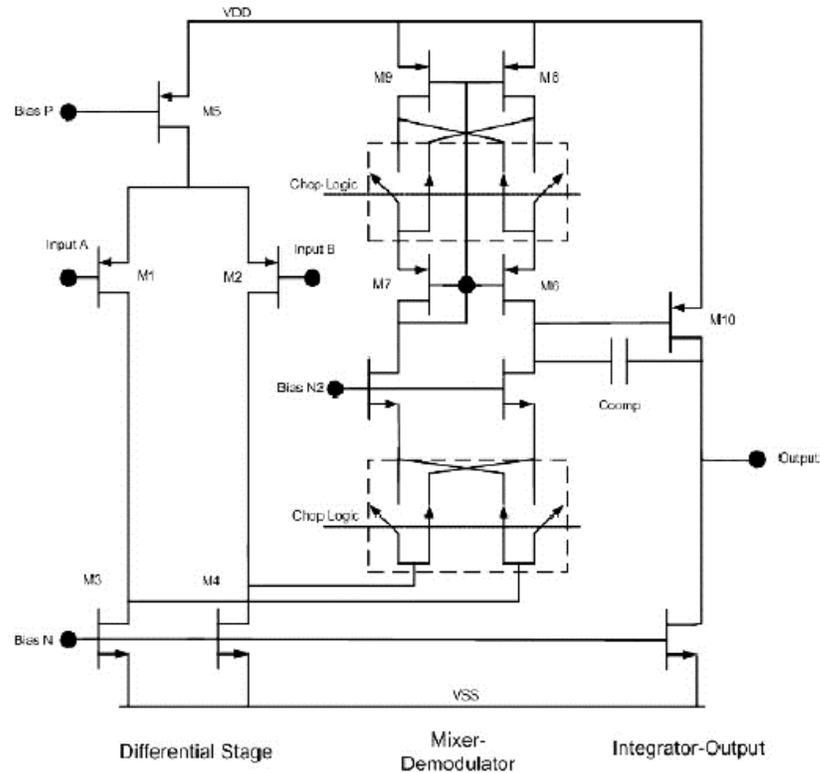
Figure 4: Addition of chopper circuit into classical folded-cascode amplifier [8]
