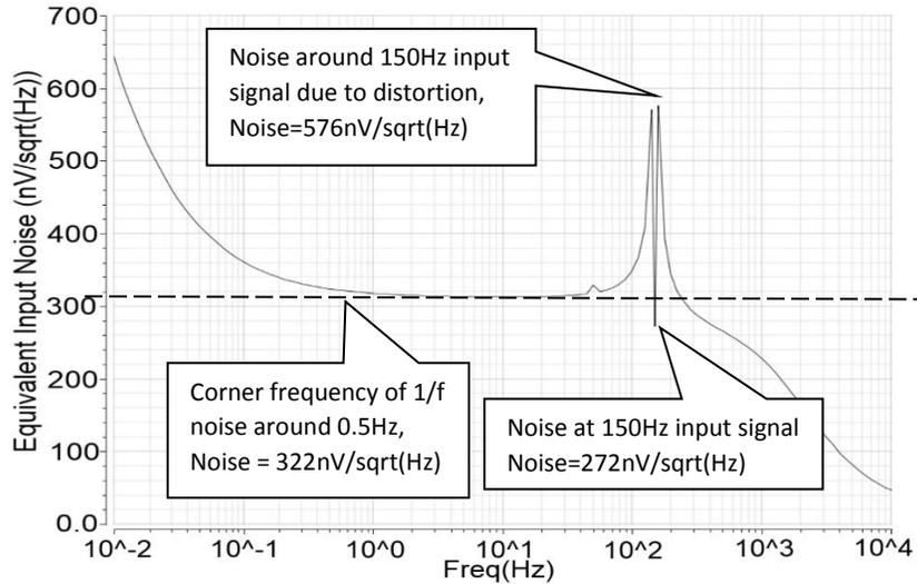
Figure 18, Noise Profile of the Proposed BPA with chopping frequency at 5kHz (input signal of 300uV at 150Hz)
