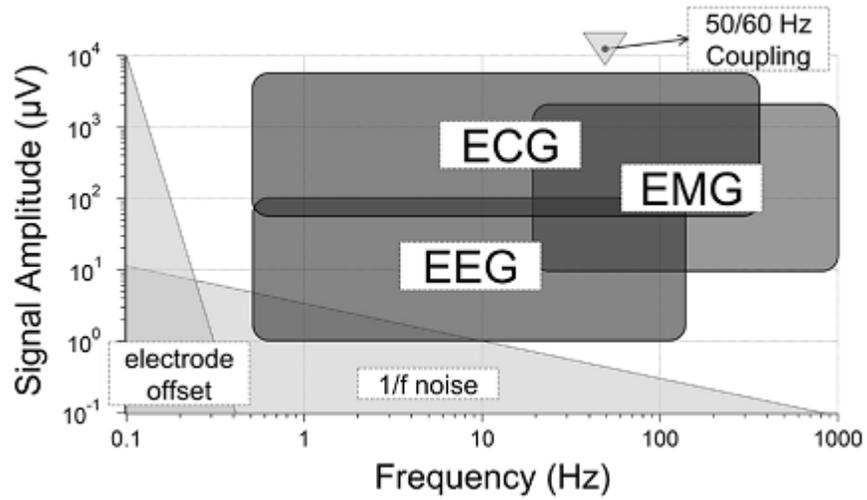
Figure 1: Characteristics of biopotential signal and nearby corrupting signals [9].
