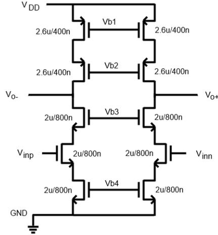
Figure 14, Telescopic Cascode Amplifier Transistor Sizing
