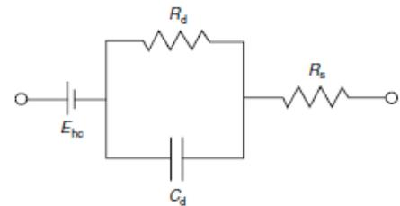
Figure 10: Equivalent Model for Electrode[1]
