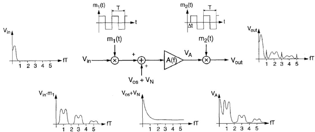
Figure 2: Principle of chopper stabilization technique (without LPF stage) [12]
