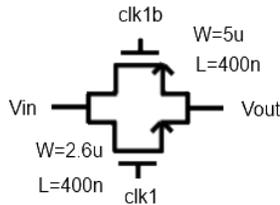
Figure 17, Complementary CMOS Switch for Charge Injection Compensation
