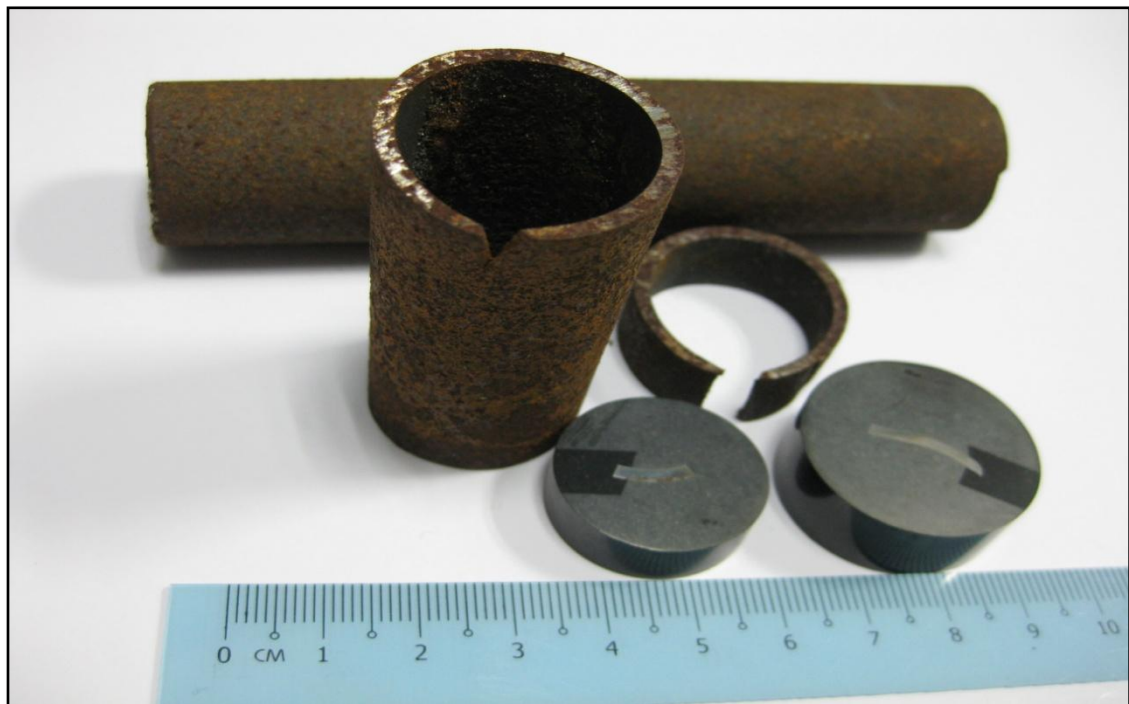
Figure 3.3: Metallographic sample preparation (failed and normal sample)
