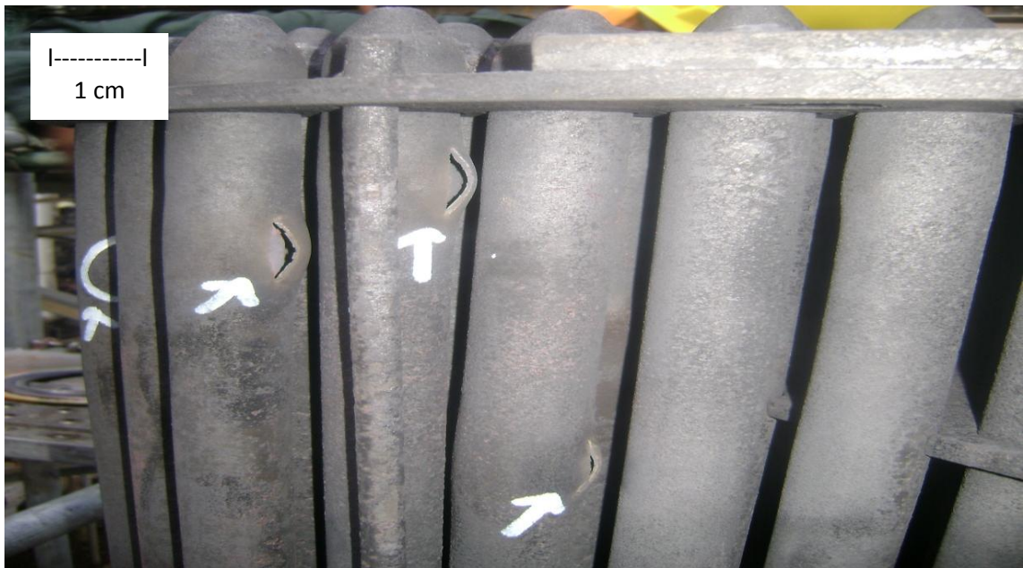
Appendix 3: Heat exchanger tube failure position
