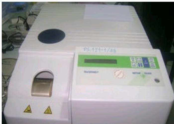
Figure 3.13: TGA Machine for proximate analysis
